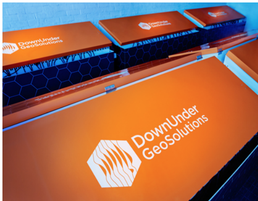
The rows of oil tanks in which the computers are suspended.
